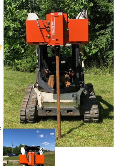
Dimensions: 21 X 12 X 4" (main body without quick mount plate) Weight: 143 LB. w/quick mount plate & tool 243 LB. w/quick
