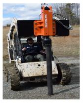
Dimensions: 40x18x12 (main body without quick mount plate) Flow: 5.5-7 GPM
